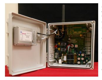
The Telescada NeXGen™ CCU-462 Wireless Capacitor Controller with integrated Raveon M7 Digital UHF Radio
