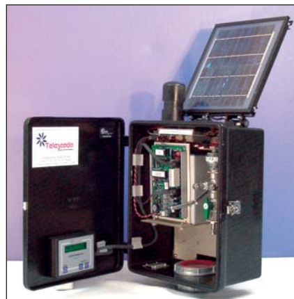
Figure 2: Photo of RTU and internal components. The cost-effective solution uses new
